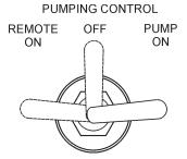
Figure 24. Pumping Control Switch (ON)
